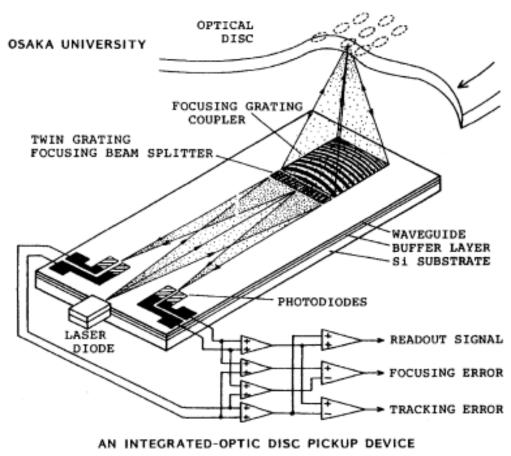
the optical readheads used in commercially available audio compact disk (CD) players often have eight or nine discrete optical elements, all of which have to be held in exact alignment in the face of much shock and vibration.
