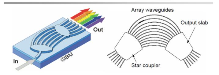
Array waveguides gratings (AWGs) are useful components for WDM networks (WDM = Wavelength Division Multiplexing).
